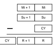
SBBL(—) can also be used to subtract signed binary data. The underflow and overflow flags (SR 25404 and SR 25405) indicate whether the result has exceeded the lower or upper limits of the 32-bit signed binary data range. Refer to page 29 for details on signed binary data.
